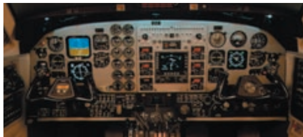
A proven winner with a reputation for rock-solid performance, the Collins Pro Line II is ergonomically designed to enhance single-pilot operation. It is available with your choice of four- or five-inch displays.
