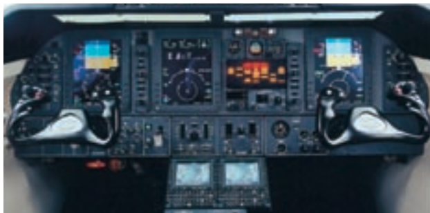
The Premier I showcases the advanced Collins Pro Line 21 avionics suite featuring two or three, easy-to-read 8" x 10" liquid crystal displays.
